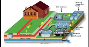
Sewage goes to a **sewage** treatment works. Sewage goes through a process of aeration to help bacteria digest waste
